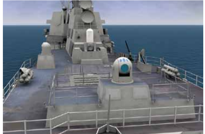
Laser weapon ship integration analyses have been performed to determine potential beam director and subsystem locations for DDG 51.
