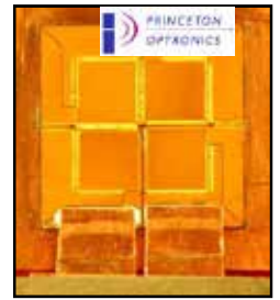
2x2 VCSEL Array 2.7x2.7mm / 530W power
